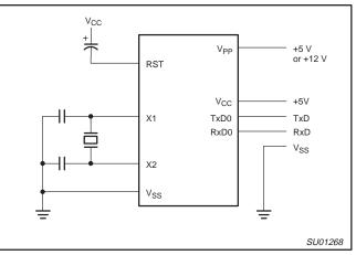
Figure 2. In-System Programming with a Minimum of Pins
